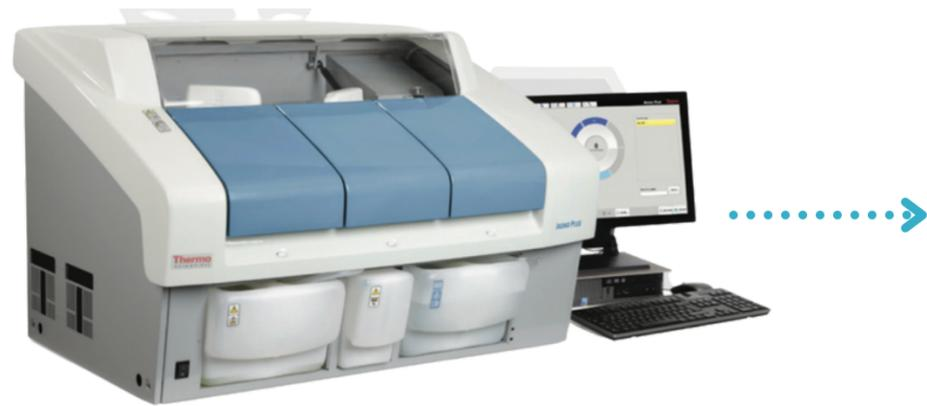
Thermo Scientific Indiko Plus is discrete cell technology that enables synchronous analysis of several different tests from the same sample, and different types of samples can be analyzed simultaneously.
